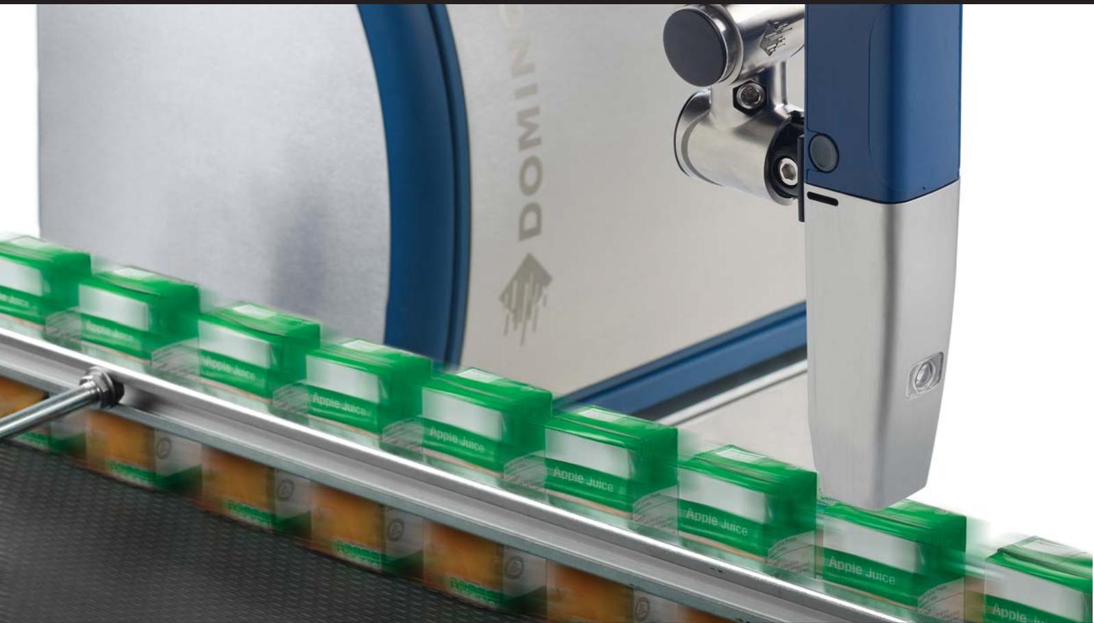
Continuous ink jet (CIJ) or small character coding is the most common method for high-speed coding of use-by dates and batch codes. Advancements in printhead design, ink formulations and preventative maintenance regimes has made continuous ink jet technology more consistent, cleaner and easier to live with than ever before.
